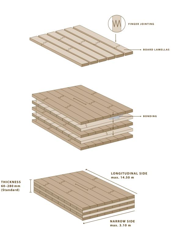
*Further explanations on the principle and layout of a PFEIFER CLT panel can be found on pages 18 and 19.*
